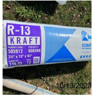
Insulation Label and R-Value
